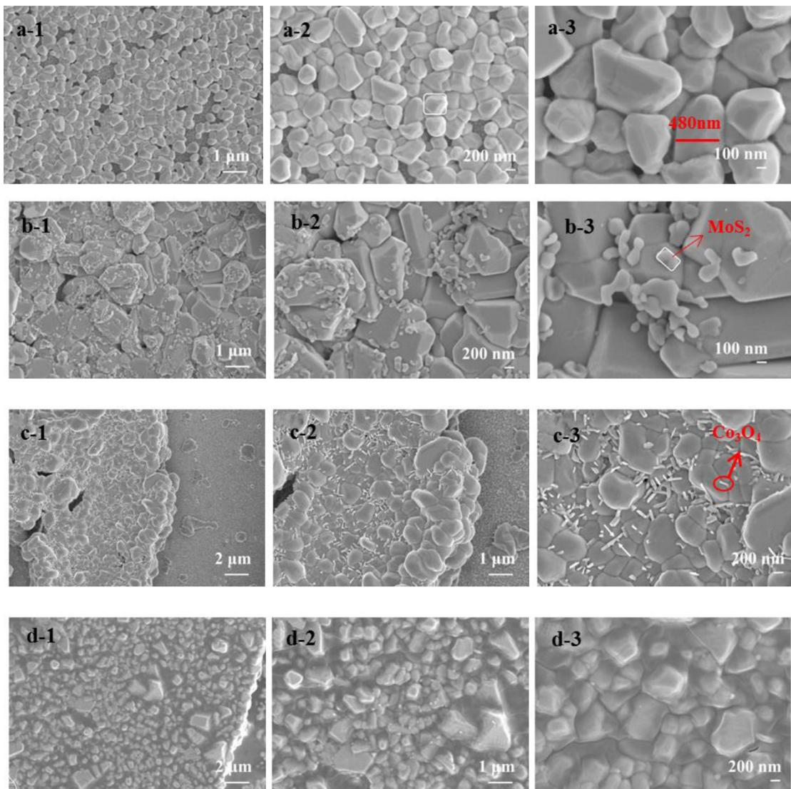
**Fig. 1 – Scanning electron microscope (SEM) images of (a) BiVO<sub>4</sub>, (b) BiVO<sub>4</sub>-MoS<sub>2</sub>, (c) BiVO<sub>4</sub>-MoS<sub>2</sub>-Co<sub>3</sub>O<sub>4</sub> and (d) electrochemically-modified BiVO<sub>4</sub>-MoS<sub>2</sub>-Co<sub>3</sub>O<sub>4</sub> (E-BiVO<sub>4</sub>-MoS<sub>2</sub>-Co<sub>3</sub>O<sub>4</sub>) films. The numbers 1, 2, and 3 refer to images with different magnification.**
