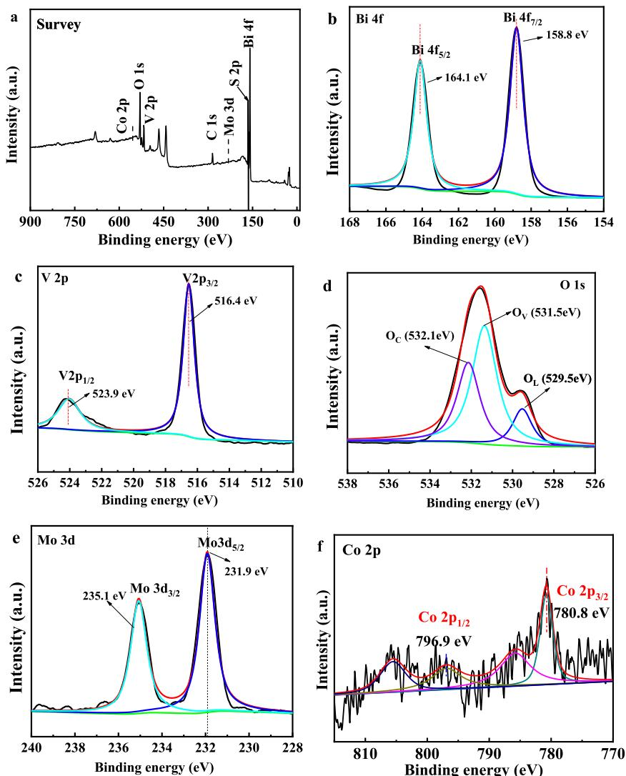
**Fig. 3 – X-ray photoelectron spectroscopy (XPS) spectra of E-BiVO<sub>4</sub>-MoS<sub>2</sub>-Co<sub>3</sub>O<sub>4</sub> film electrode (a) survey spectrum and high-resolution core spectrum for (b) Bi 4f, (c) V 2p, (d) O 1 s, (e) Mo 3d, and (f) Co 2p.**
