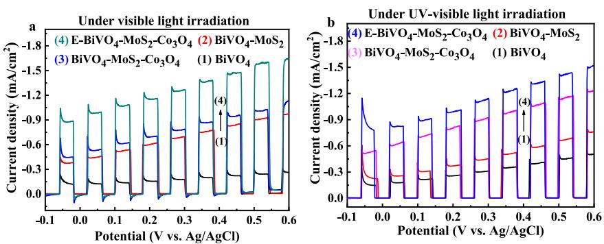
**Fig. 4 – Linear sweep voltammetric curves of BiVO<sub>4</sub>, BiVO<sub>4</sub>-MoS<sub>2</sub>, BiVO<sub>4</sub>-MoS<sub>2</sub>-Co<sub>3</sub>O<sub>4</sub> and E-BiVO<sub>4</sub>-MoS<sub>2</sub>-Co<sub>3</sub>O<sub>4</sub> films under (a) chopped visible and (b) UV-visible light irradiation in 0.1 mol/L NaOH aqueous solution.**
