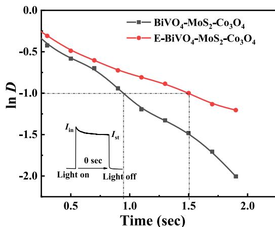
**Fig. 5 – Normalized plots of photocurrent as a function of time for different as-prepared films. Inset: typical photocurrent transient response curve at 0.5 V (vs. Ag/AgCl).  $I_{in}$ : photocurrent was measured at irradiation time of 0 sec;  $I_{st}$ : photocurrent obtained at steady state;  $D$ : transient photocurrent.**
