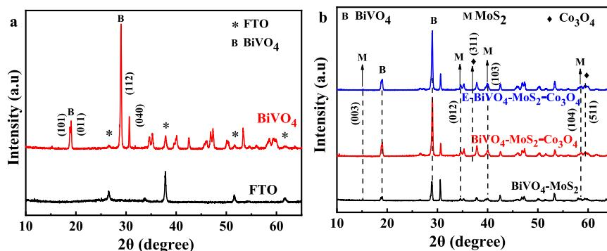
**Fig. 2 – X-ray diffraction (XRD) patterns of (a) FTO, BiVO<sub>4</sub> and (b) BiVO<sub>4</sub>-MoS<sub>2</sub>, BiVO<sub>4</sub>-MoS<sub>2</sub>-Co<sub>3</sub>O<sub>4</sub> and E-BiVO<sub>4</sub>-MoS<sub>2</sub>-Co<sub>3</sub>O<sub>4</sub> films.**
