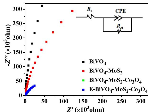
**Fig. 6 – Nyquist plots of  $\text{BiVO}_4$ ,  $\text{BiVO}_4\text{-MoS}_2$ ,  $\text{BiVO}_4\text{-MoS}_2\text{-Co}_3\text{O}_4$  and  $\text{E-BiVO}_4\text{-MoS}_2\text{-Co}_3\text{O}_4$  films under dark condition in 0.1 mol/L NaOH aqueous solution. The inset shows the equivalent circuit using to fit the Nyquist plots.  $Z''$ : imaginary impedance;  $Z'$ : real impedance;  $R_s$ : series resistance;  $R_{ct}$ : interface charge transfer resistance; CPE: constant phase angle element.**
